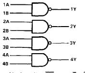
positive logic;  $Y = \overline{A \cdot B}$  or  $Y = \overline{A} + \overline{B}$
